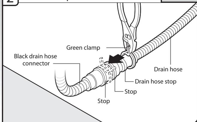
Using pliers, squeeze open the small green drain hose clamp and slide onto connector between stops.
